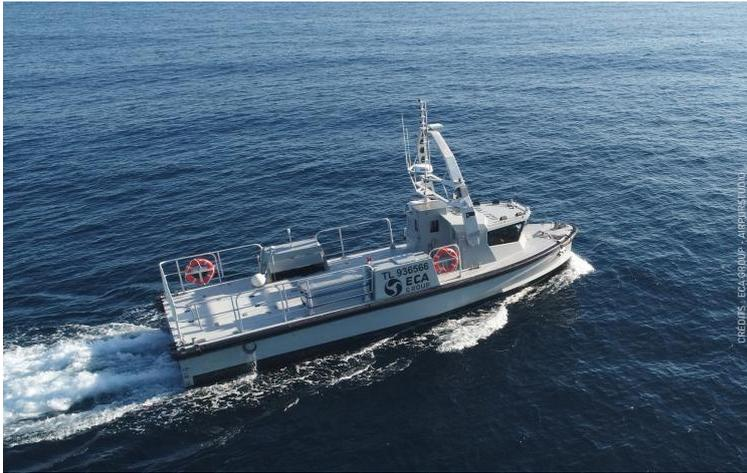
**Figure 6: Drone de surface 12 ml (source ECA Group)**
