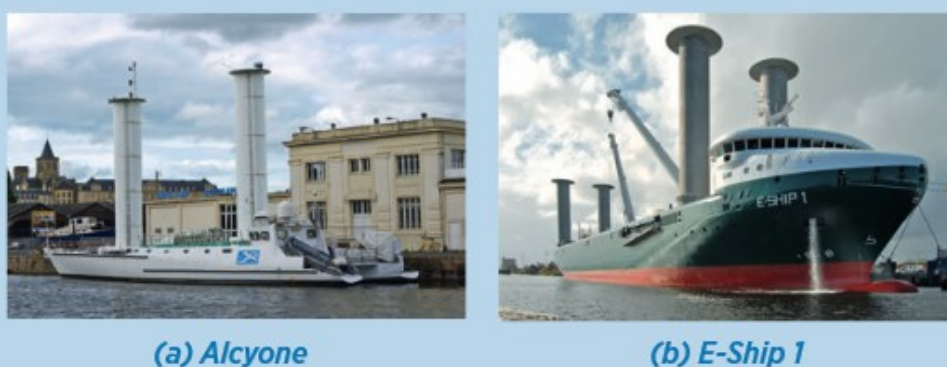
Figure 4: Ships using rotor sail (Magnus Effect)
